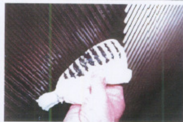
Aifa-laval exchanger Quench water side Mat polymeric sediments may be removed from plate surface by soft paper.
